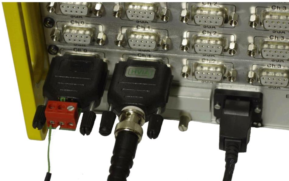
THIA- and HVIA Input Adapter connected to a Traveller CF-System
